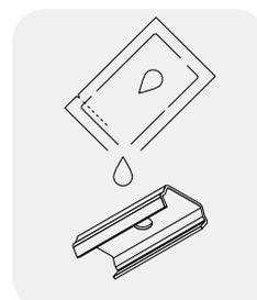
Lubricate (B) clips using the silicone grease provided (E).
